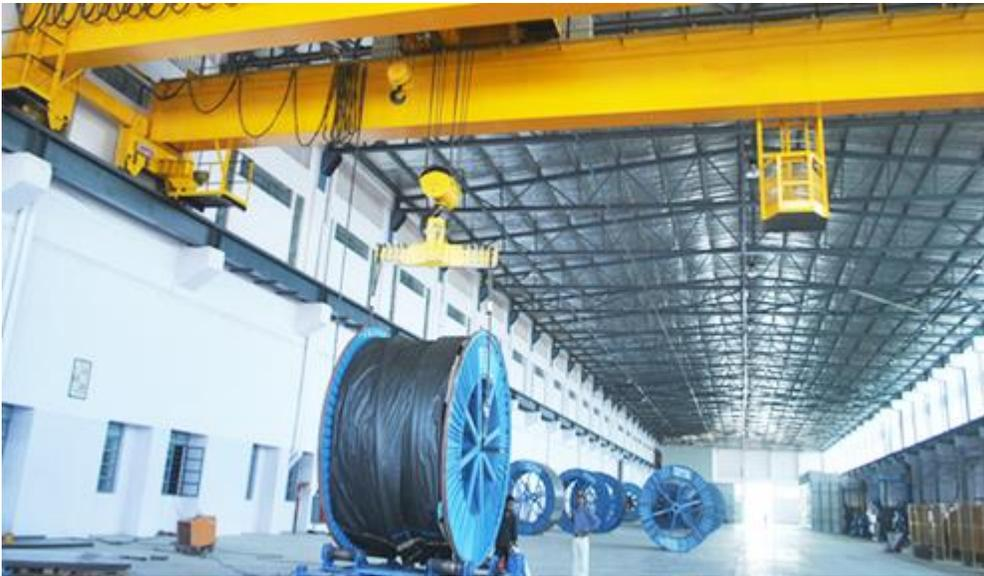
Crane capacity upgradation can save over 50% of cost as compared to replacement of existing crane by new. However, Crane upgradation needs high degree of understanding of crane design and analytical ability to carry out accurate reverse engineering. In most of the cases manufacturing drawings of existing crane are not available with the crane user and in such a situation detailed study of existing crane is essential to determine its suitability for capacity/ span upgradation.
