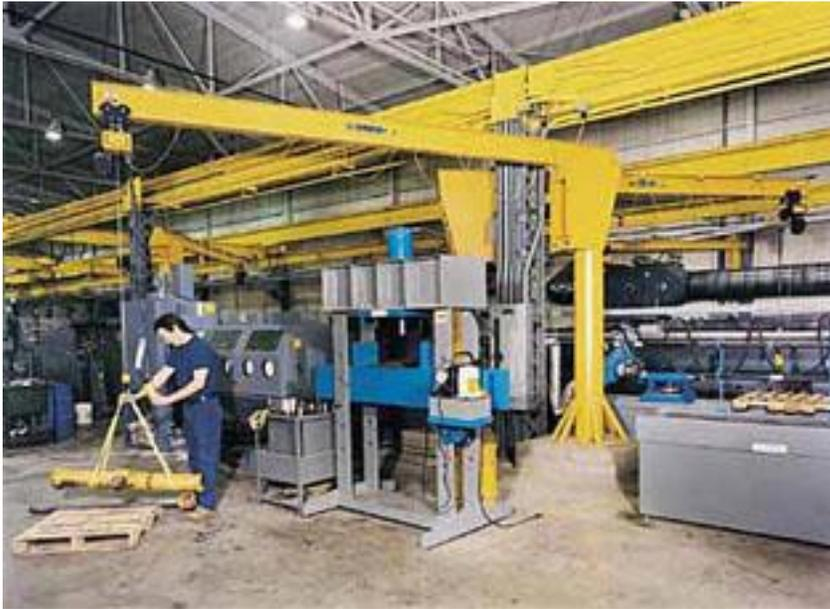
Pillar mounted (Free Standing) Jib Cranes are best suited for work station application. These cranes are directly installed on shop floor without any need for support from building column. Available in capacity ranging from 0.5 MT to 5 MT and outreach of 8 meters, these cranes serve the need of local station without use of shop EOT Crane.
